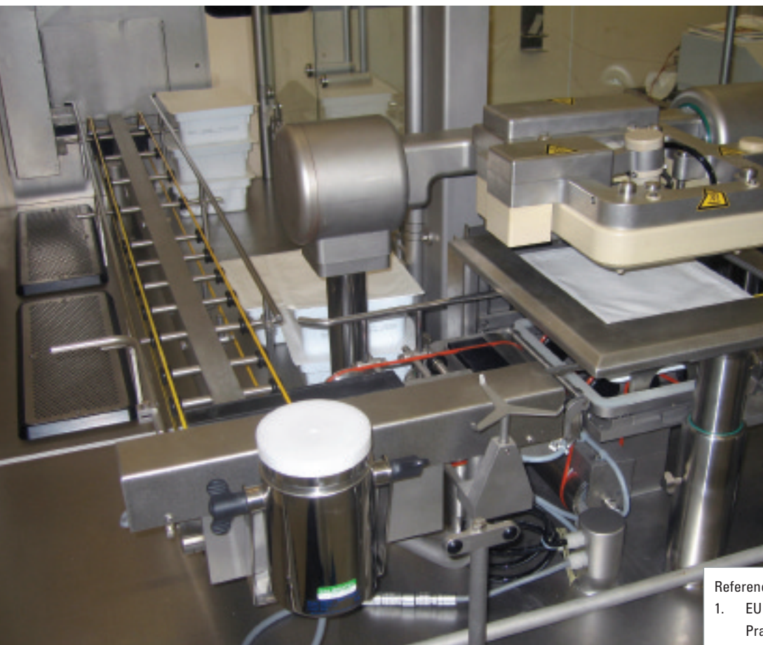
Figure 3: Remote control microbiological air samplers can be bespoke to each filling line
